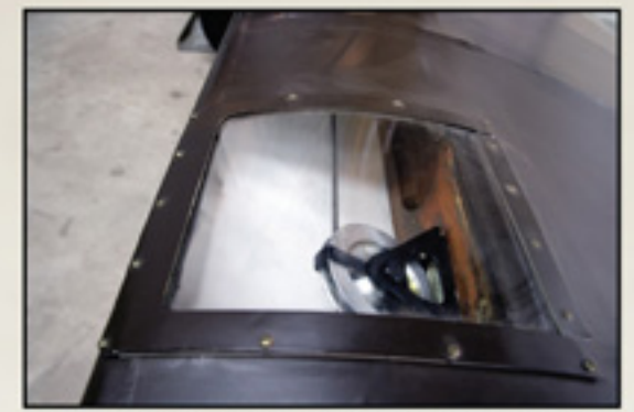
Pulley inspection panel detail from Shuttleworth's Sopwith Pup. (converted from a Sopwith Dove)
