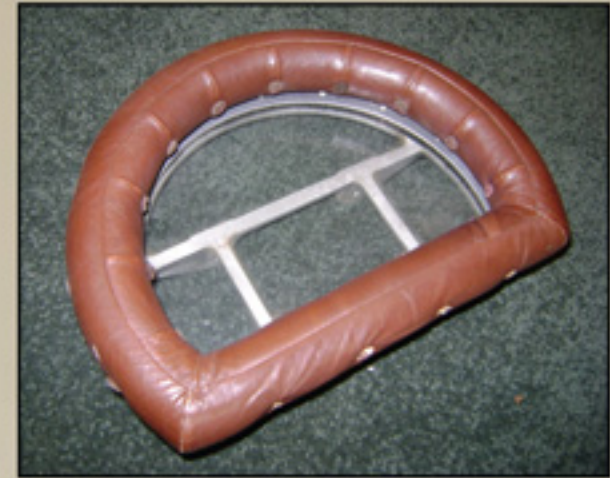
Sopwith pattern Vickers Gun padded windscreen.
