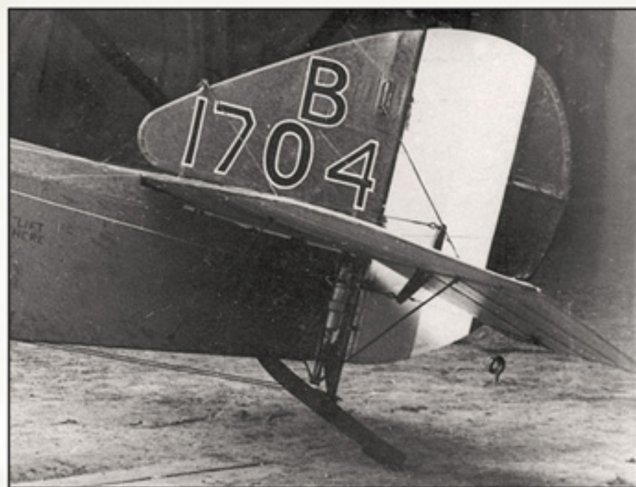
Adjustable tailplane detail from Standard built Pup B1704.
