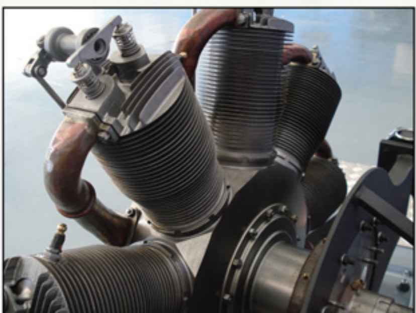
LeRhone 9c 80hp engine. Note the copper intake header assemblies.
