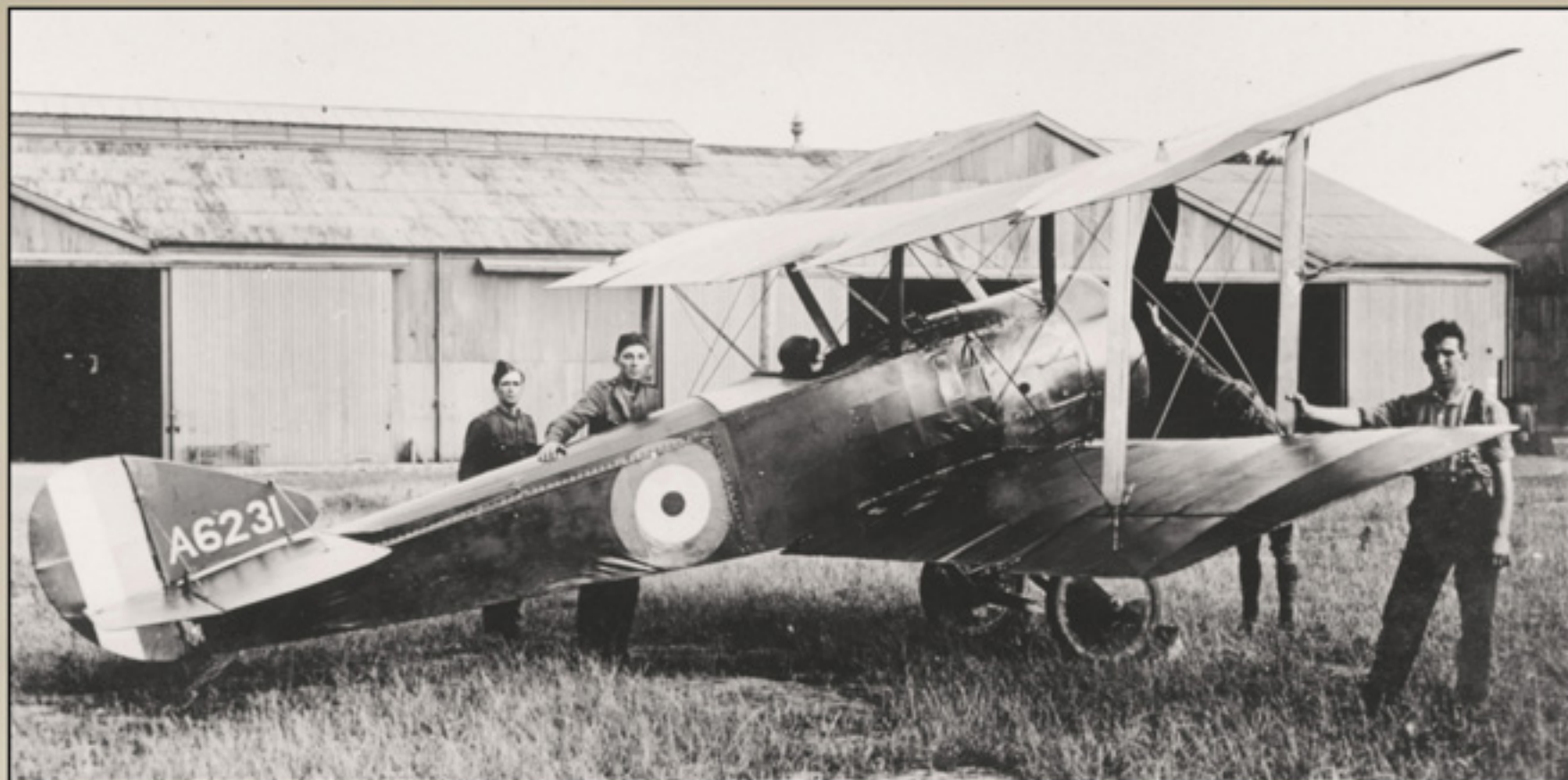
Whitehead built Pup A6231 of 63 TS (Training Squadron) at Joyce Green mid 1917. Note the fixed tail plane and lack of armament.
