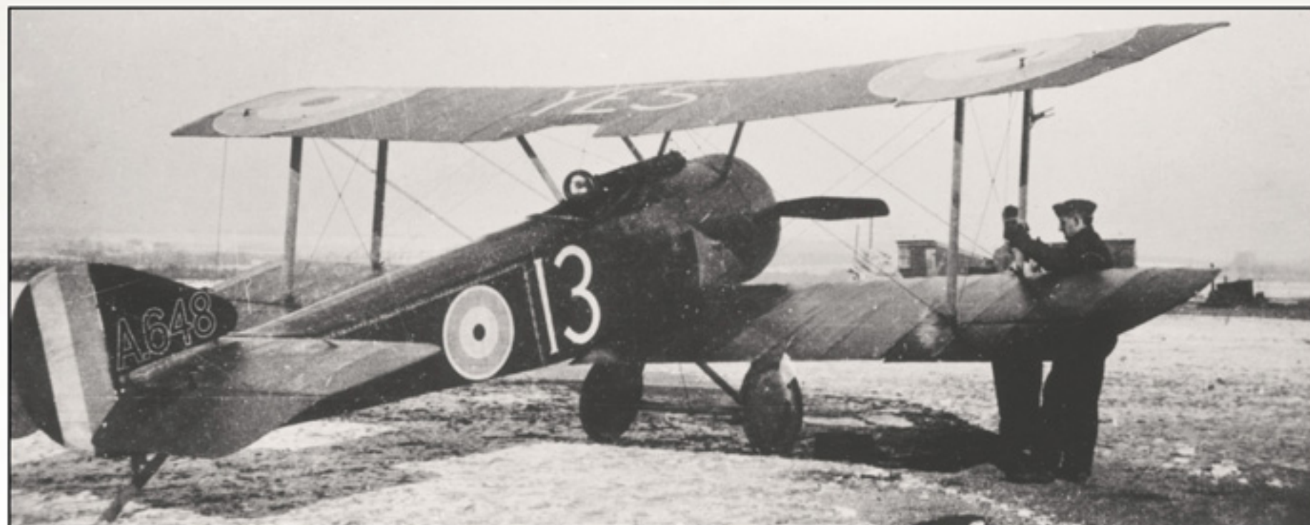
Standard built Pup A648 'YES' shown in the markings of 54 Sqn December 1916. It has an adjustable tailplane and Sopwith padded Vickers Gun windscreen.
