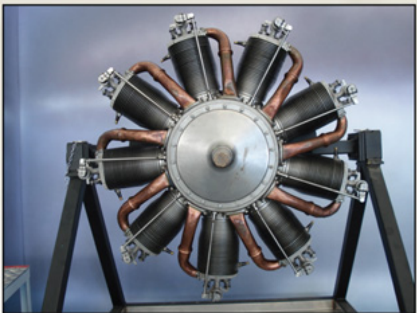
LeRhone 9c 80hp engine. Note the copper intake header assemblies.
