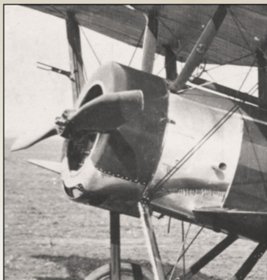
Flat faced cowling shape peculiar to Pups built by the Standard Motor Co Ltd.
