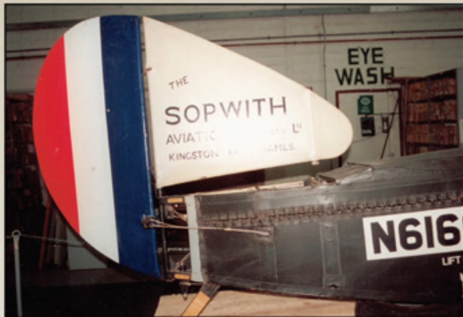
Sopwith Pup replica N6160 displays the general arrangement of its fixed tail plane fittings. (Photo by David Frowen)
