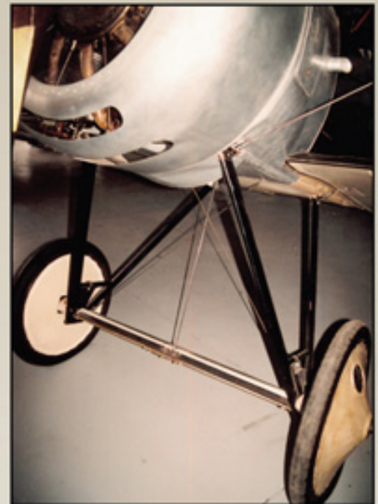
Undercarriage detail from Sopwith Pup replica N6160. Note that it is not typical for the split axle to be flat as shown here unless the aircraft is in flight, they should angle upwards under the weight of the aircraft as shown elsewhere. (Photo by David Frowen)
