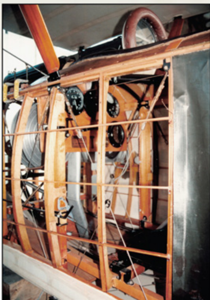
The very accurate Sopwith Pup replica N6160, built by EMK Aeroplanes Ltd/Skysport Engineering from 1978 to 1983, undergoing repairs at the RNZAF museum. Note the various wood tones, CDL fuselage wall interior and the empty belt winder drum for the Vickers Gun. (Photos by David Frowen)
