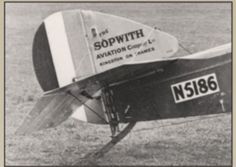
Adjustable tail plane detail from Sopwith built Pup N5186.
